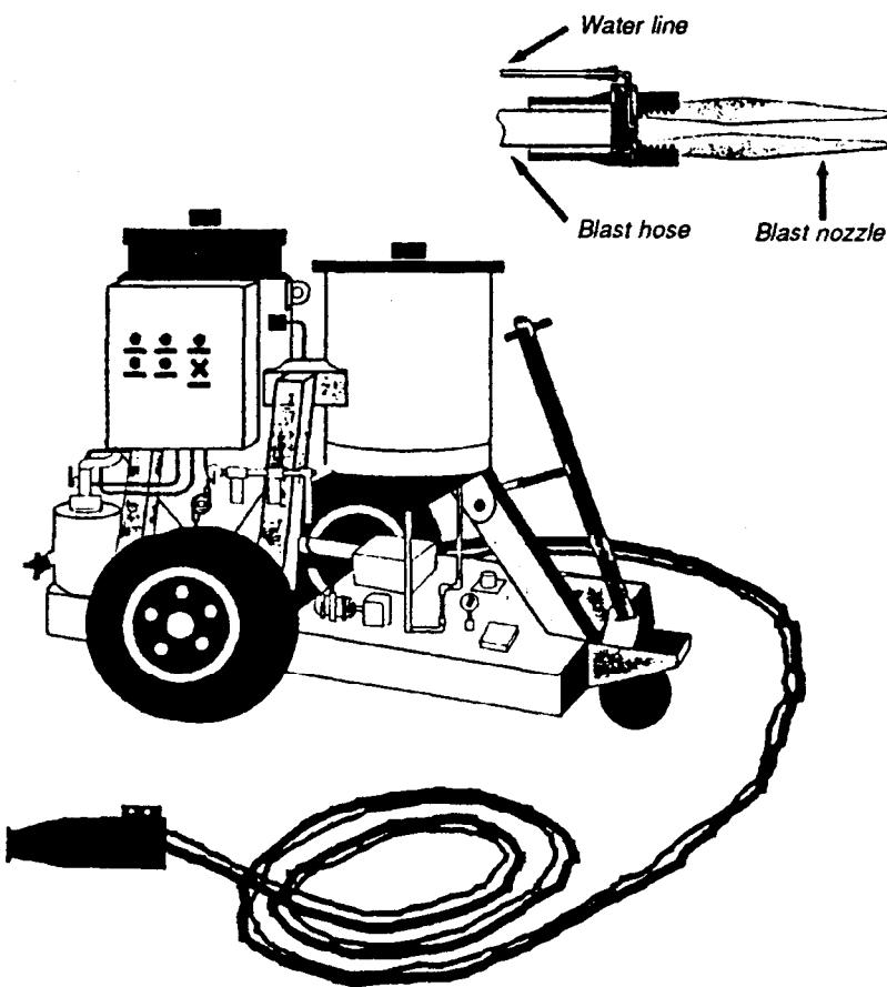
Figure 1. ACCUSTRIP SYSTEM™ with wet blast head.
