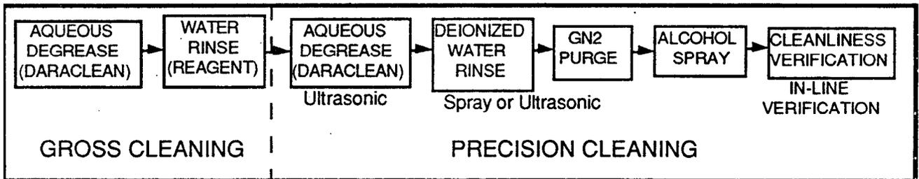
FIGURE 1 Current Precision Cleaning Method
