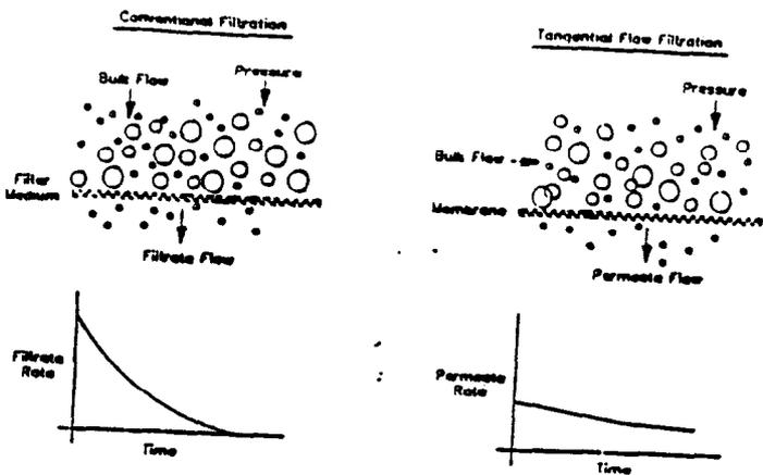
Fig. 1: Comparison of Flow Patterns
