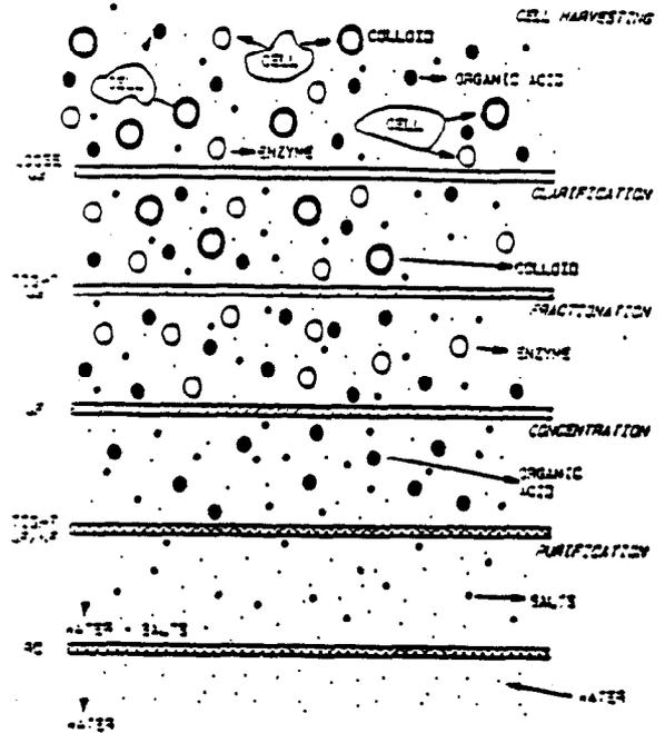
Fig. 2: Membrane Filtration Concepts
