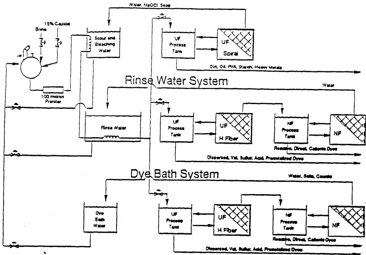
Fig. 9: Full Recycle of Jet Dyeing Machine Waters
