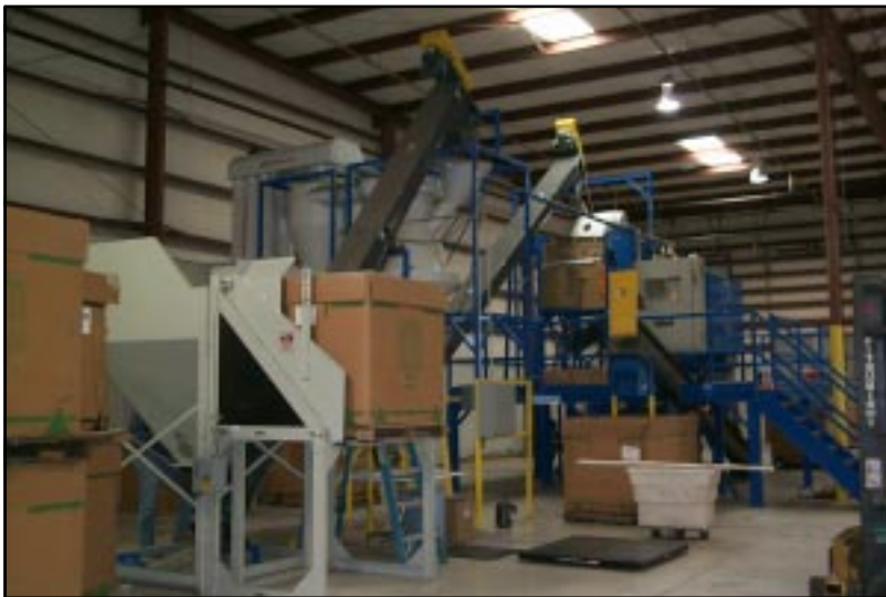
The PET/PVC flake sorter system depicted above reduces PVC contamination to less than 200 parts per million.
