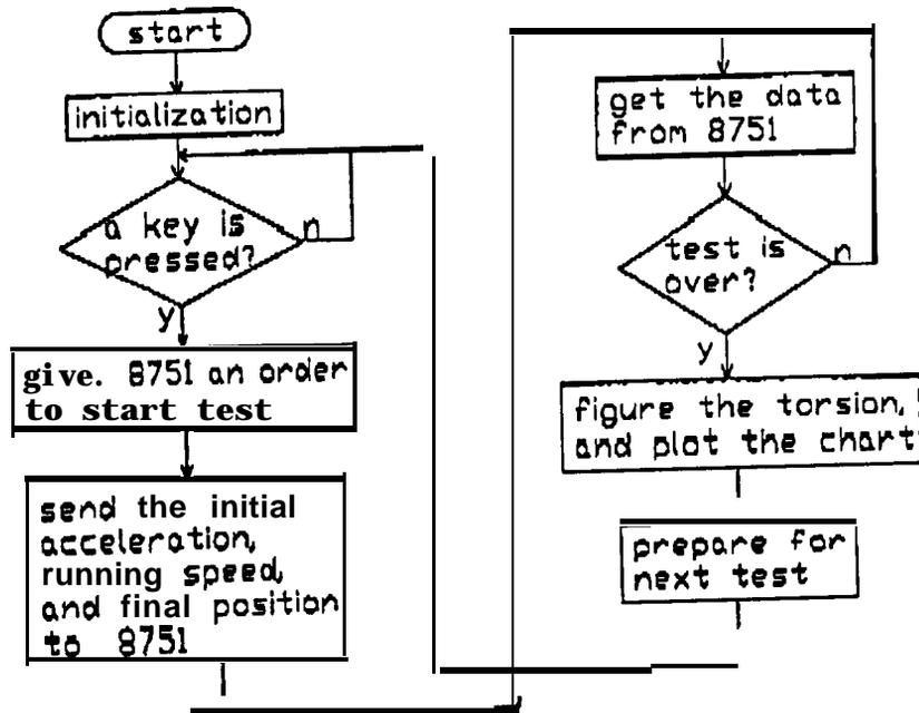
Figure 3, software for main computer
