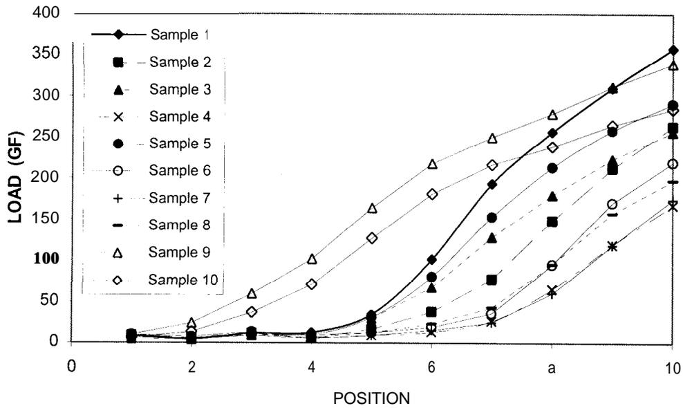
Figure 3. Load at different position of compression cycle
