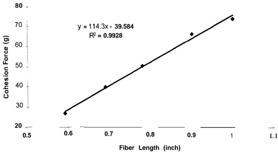
Figure 7. Cohesion force of cotton fibers vs. fiber length
