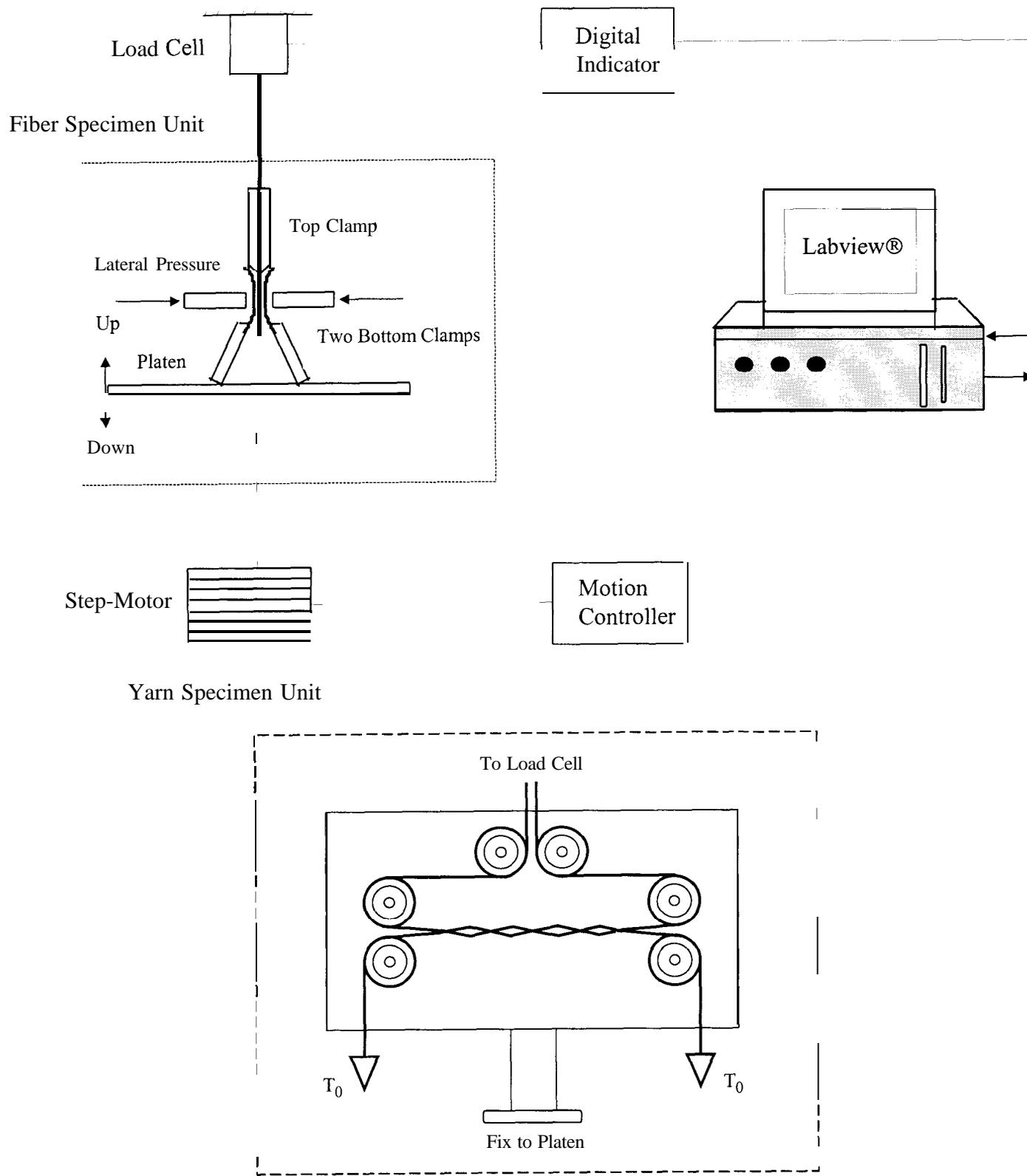
**Figure 1.** A schematic diagram of Auburn Beard Test Instrument
