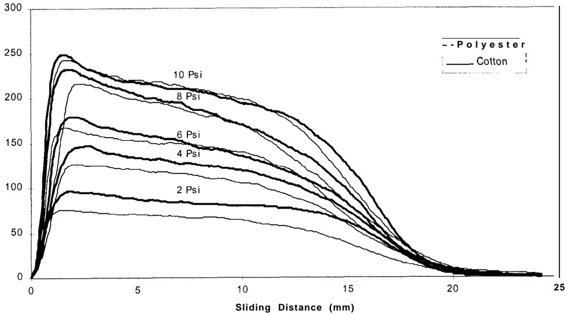
**Figure 4.** Friction profiles of cotton and polyester fibers obtained using Auburn Beard Test
