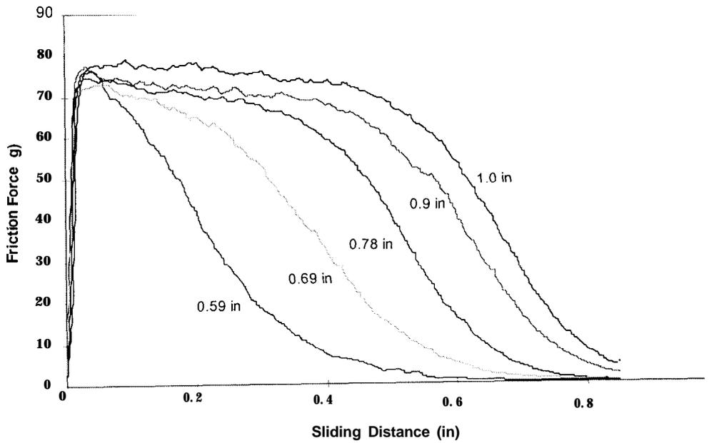
Figure 6. Friction profiles of cotton fibers at different fiber length
