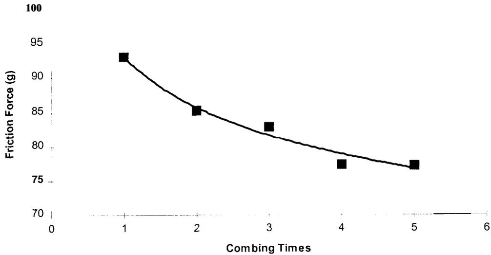
**Figure 5.** The maximum friction force vs. the HVI combing times for cotton fiber
