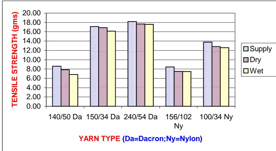
Figure 6. Individual filament strength test
