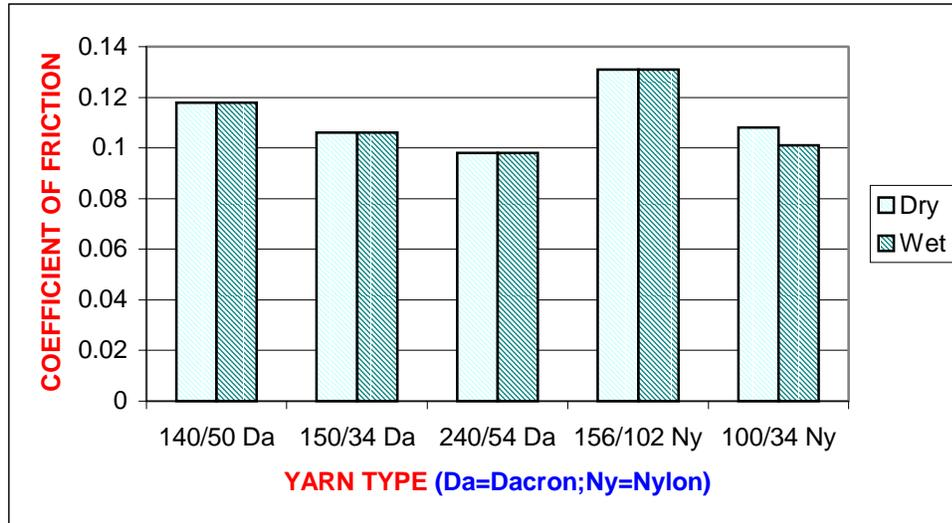
Figure 4 Yarn to Yarn Friction
