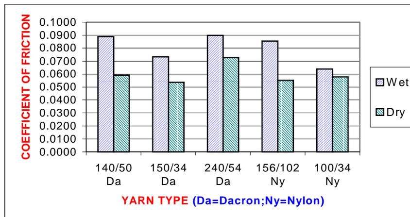
Figure 3 Yarn to Metal Friction
