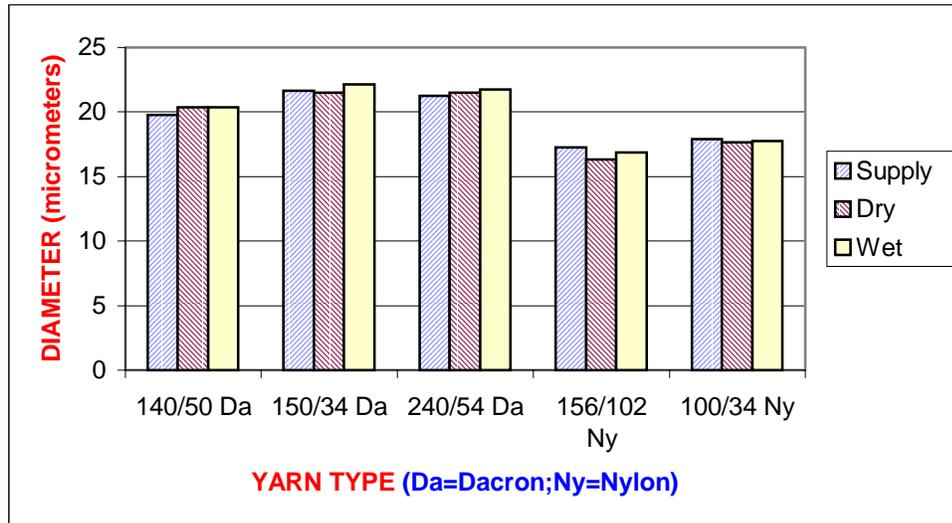
Figure 2. Filament diameter Measurements
