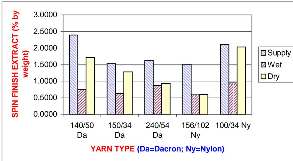
Figure 5. Spin finish measurements
