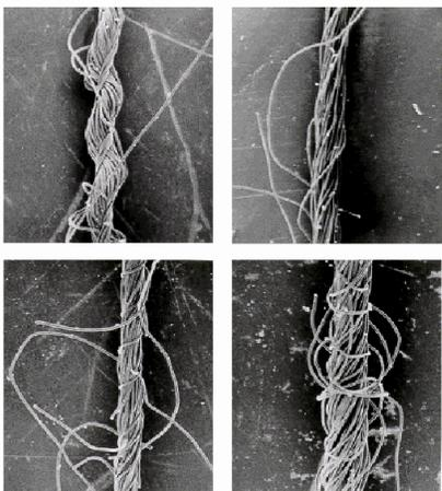
Figure 7. Jet spun yarn structure
