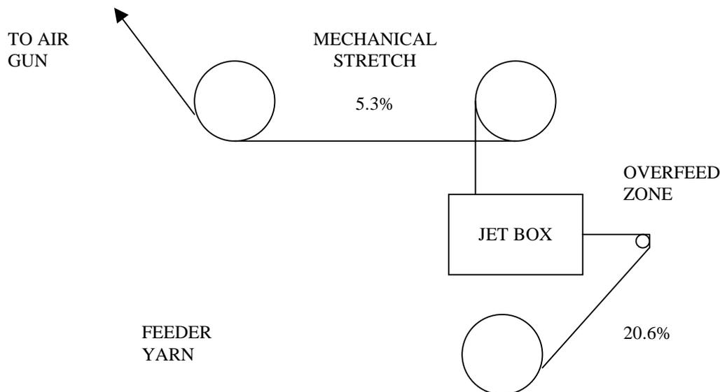
Figure 1. Experimental setup at NCSU, College of Textiles
