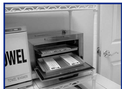
One kind of autoclave that is used to sterilize nail care instruments
