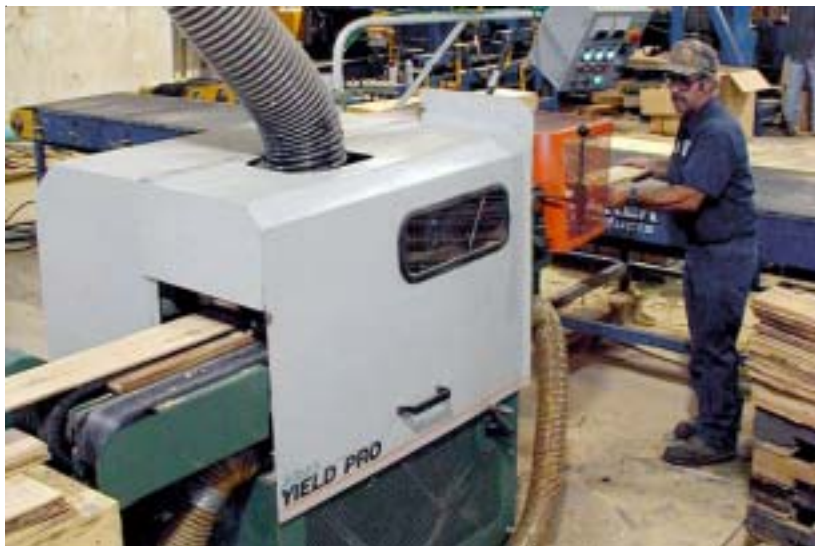
Pallets-to-flooring board milling.
