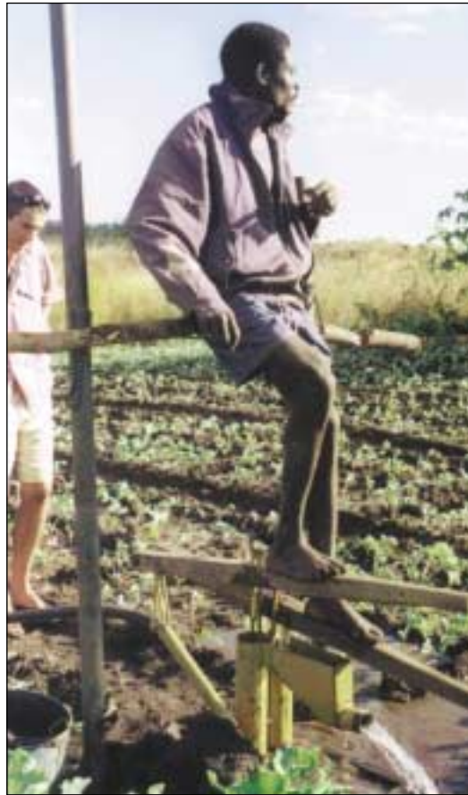
Figure 6 This pump had a seat added so the wife can use it when he is marketing
