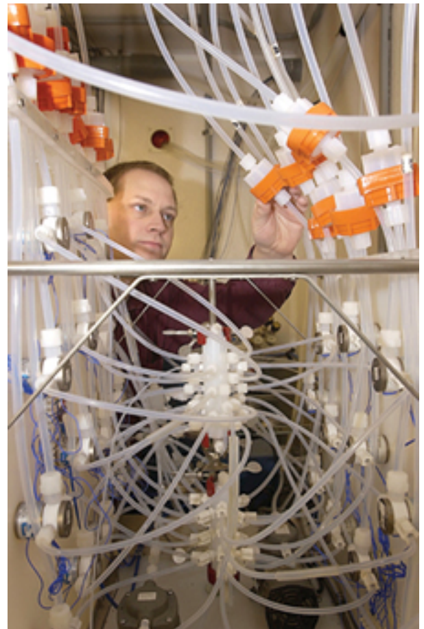
A mass of hoses and wires helps researchers like Brian Richert monitor the air quality at an animal research center located northwest of Purdue University campus. This is a sample of the equipment and process that researchers will use to study livestock air emissions.
