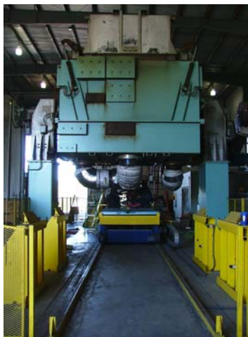
Materials are loaded into AMP's RODECS oven (above) for cleaning and decoating.
